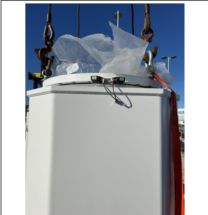
2751 – Sensor and stops on Pedestal base Ring
