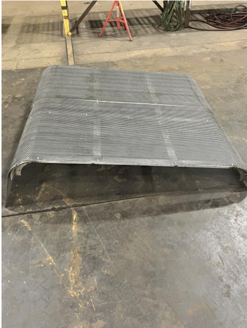
5167 – Heat Shield being made ready for installation
