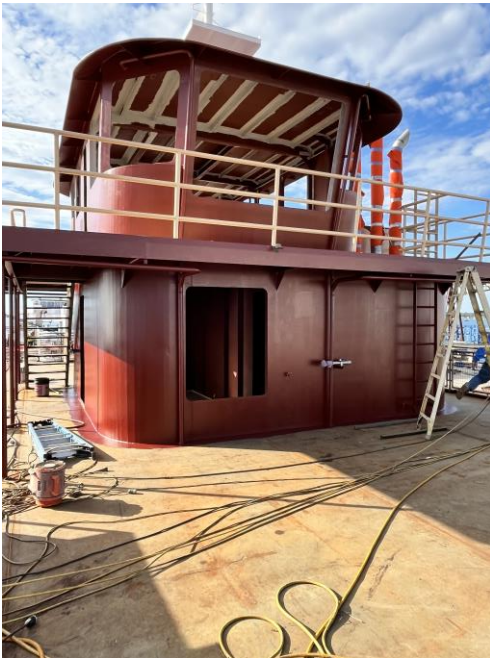
5170 – PH and Electrical Equip Room and Crew Locker Painted
