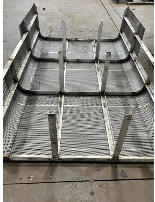
5168 - Heat Shield being made ready for installation
