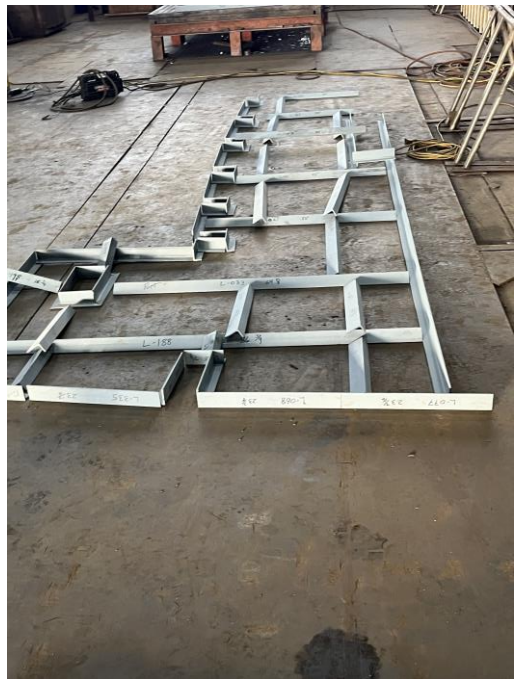
5230 - Equipment Foundation Framing Components
