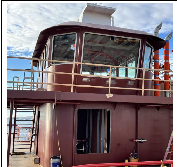
5377 – PH with Windows – Still Need Wipers Installed
